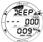
Fig. 85 - DELAYED VIOLATION #3 MAIN
