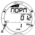
Fig. 3 - LOW BATTERY WARNING
