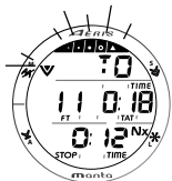
Fig. 83 - DELAYED VIOLATION #1 MAIN
