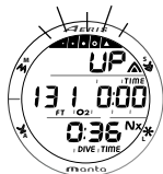
Fig. 25 - O2 EX- CEEDED
