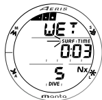
Fig. 32 - NORM SURFACE MODE (Post Dive Wet)
