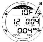
Fig. 78 - DECO STOP MAIN
