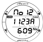
Fig. 91 - LOG PREVIEW (during Transition Period)
