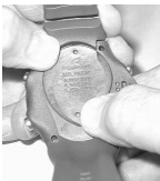
Fig. 118 - BATTERY HATCH REMOVAL (without tool)
