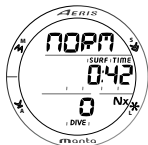
Fig. 31 - NORM SURF MAIN (no dive made)
