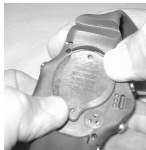
Fig. 123 - BATTERY HATCH O-RING (without tool)
