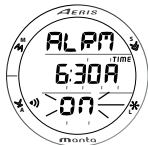
Fig. 21 - DAILY ALARM STATUS
