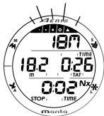
Fig. 84 - DELAYED VIOLATION #2 MAIN
