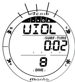
Fig. 115 - FREE SURF VIOLATION (DECO)
