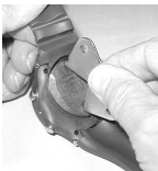
Fig. 117 - BATTERY HATCH REMOVAL (using tool)
